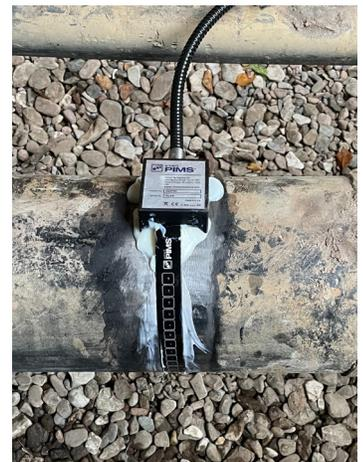
Figure 4: matPIMS™ 1x15 array permanently installed using viscoelastic putty to overcoat sensor strip and head before wrapping/backfill.
