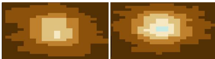
Figure 13 MFLi 14 image of defects: clearly different geometries.
