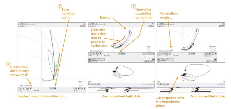
frequency to compensate for magnetic permeability differences between the calibration standard and the tubes in the bundle.
