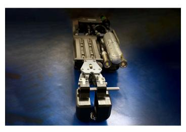
The first end effector was used to scrape or rake foreign objects like bolts from behind the baffle plate while the second end effector was used to pick up and capture foreign objects from the bottom of the pool. The remotely operated crawler was designed to pick up items smaller than 25.4 millimeters high by 63.5 millimeters wide by 63.5 millimeters long (1 inch by 2.5 inches by 2.5 inches) weighing less than 0.9 kilograms (2 pounds), all within the parameters of this application.
